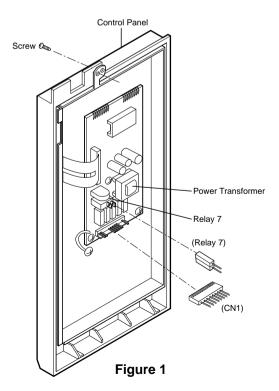
(4) Remove 3 screws securing the circuit board.
